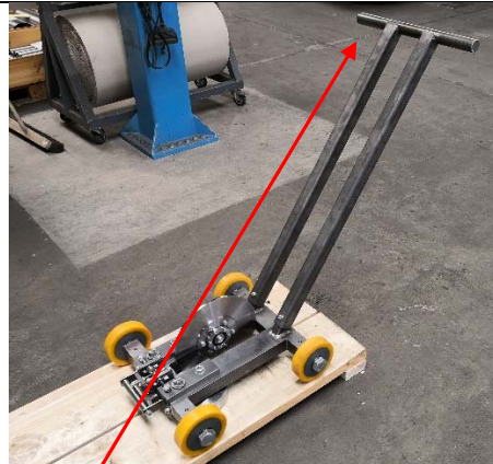
Handle for easy pushing forward of machine or easy lift up of front axis and push-in disc, demountable
