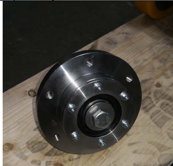
Empty Lower part of clamp holder of push-in cylinder
