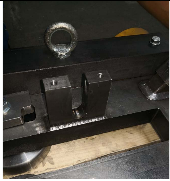
Empty Lower part of clamp holder of push-in cylinder
