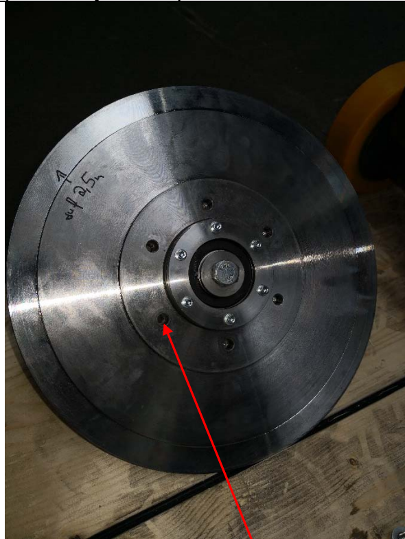
Loose outer ring screws and remove push-in disc from disc holder
