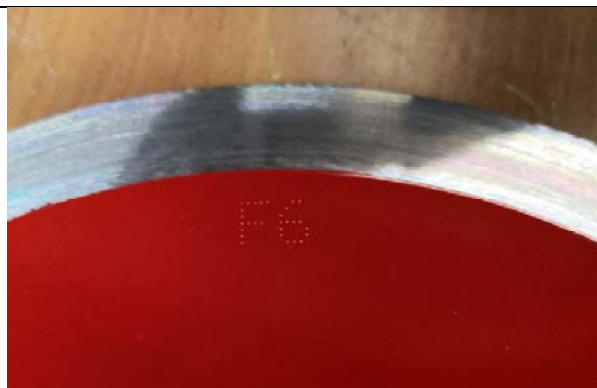
Push-in disc F6: 2,5 mm thick
