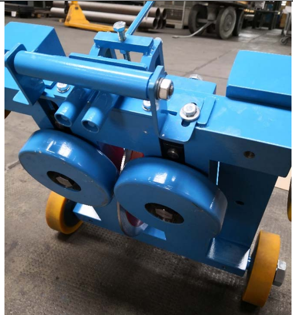
Underside of machine, guide rolls, press rolls, push-in disc
