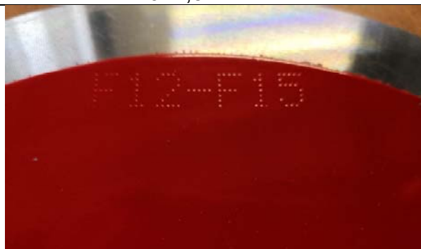
Push in disc F12 – F15: 8,5 mm thick
