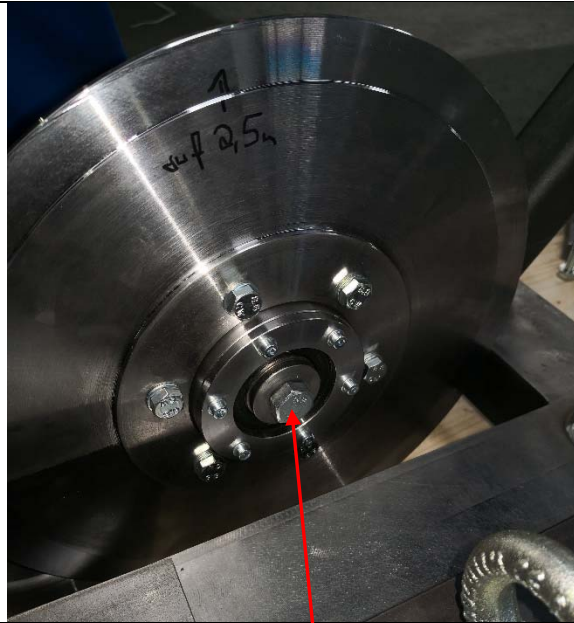
Loose center screw and lift the whole push-in cylinder upwards
